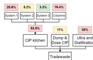
**3. Tracking of Water Flows:** Quantified the mass balance of water flows in and out of the LF plant. Provided insight into water use to formulate water saving recommendations
