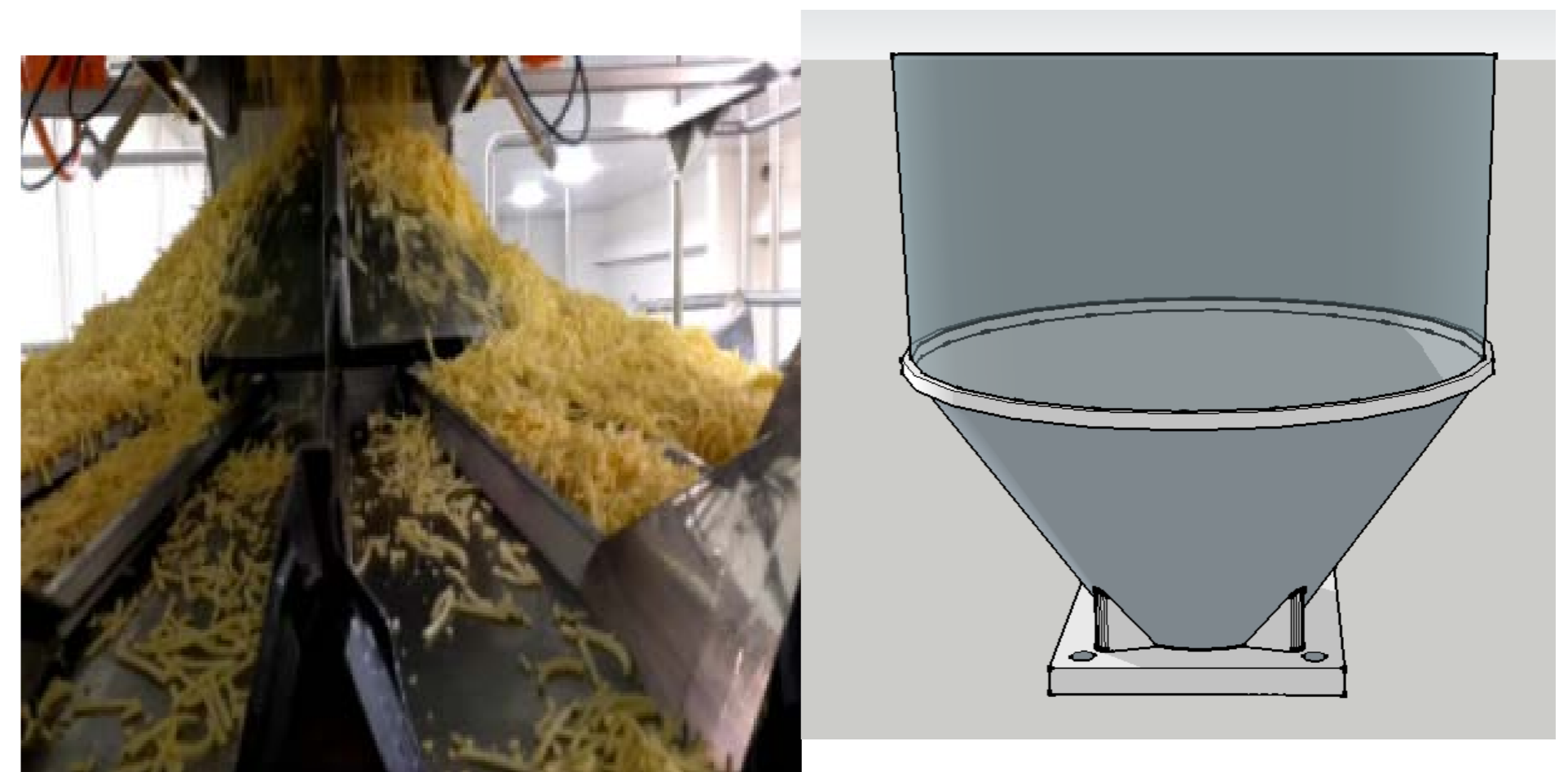
Figure 2: Hopper designed to improve cheese distribution on Ishida Multi-head weigher.
